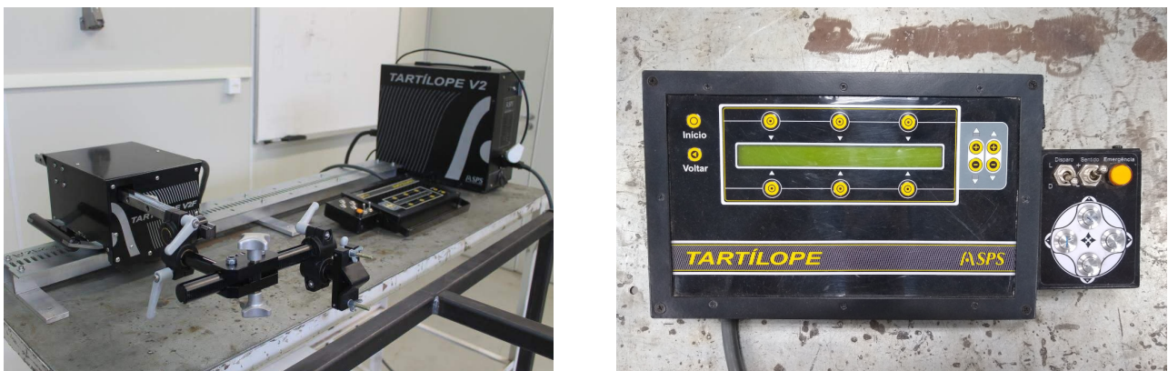
Figure 1: The Tartílope V2 (left) and its original HMI shown in detail (right).
